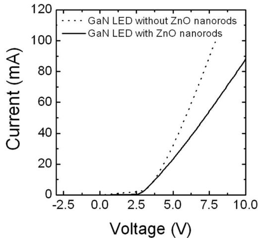
FIG. 4.  $I$ - $V$  curves of LEDs with and without ZnO nanorods. Both  $I$ - $V$  curves of the LEDs with and without ZnO nanorods exhibited nonlinear and good rectifying behavior with a turn-on voltage of 2.8 V and a leakage current of  $1 \times 10^{-5}$  A at  $-5$  V. However, series resistance of the GaN LEDs increased from 50 to 83  $\Omega$  after ZnO nanorod growth.
