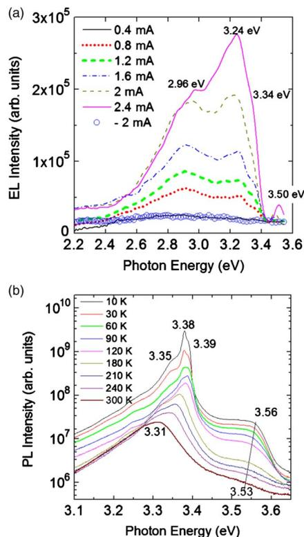
FIG. 3. (Color online) (a) Room temperature EL spectra of a  $n$ -GaN/ZnO coaxial nanorod array on  $p$ -GaN heterojunction device at various applied current levels. (b) Temperature-dependent PL spectra of GaN/ZnO coaxial nanorods.
