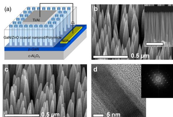
FIG. 1. (Color online) (a) Schematic illustration of a GaN/ZnO coaxial nanorod heterostructure on *p*-GaN. (b) FEG-SEM image of ZnO nanoneedle arrays grown on *p*-GaN. ZnO nanoneedles are well aligned perpendicular to the *p*-GaN surface. (c) SEM image of GaN/ZnO coaxial nanorod heterostructure. (d) HR-TEM image of GaN/ZnO coaxial nanorod heterostructures.
