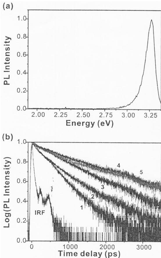
FIG. 1. Room-temperature PL spectra (a) and the TRPL measured at 3.26 eV (b) of the ZnO nanorods grown on  $\text{Al}_2\text{O}_3(00\cdot1)$ . The numbers in (b) correspond to the sample numbers in Table I. Instrumental response function of the TRPL apparatus is also shown.
