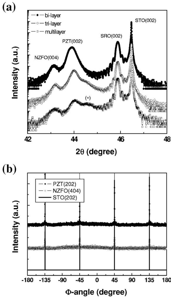
FIG. 1. (a)  $\theta$ - $2\theta$  XRD patterns of three distinct layered structures in descending order: a PZT/NZFO bilayer (180 nm), a PZT/NZFO/PZT trilayer (210 nm), and a PZT/NZFO multilayer structure consisting of 11 alternating layers (450 nm). (b) XRD  $\Phi$ -scan spectra of the 180-nm-thick PZT/NZFO bilayer.
