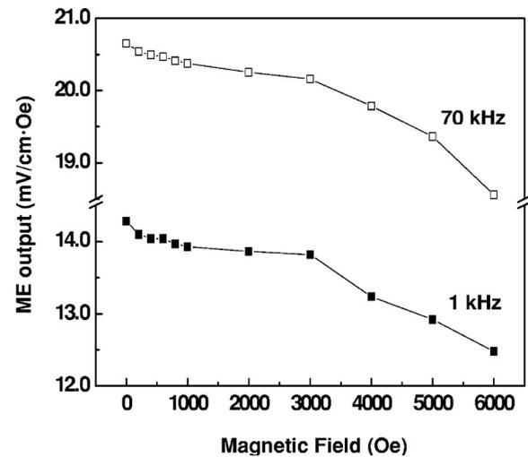
FIG. 4. Longitudinal ME voltage susceptibility values obtained by "dynamic" ME measurements at  $\omega_m=1$  and 70 kHz with the amplitude of an oscillating magnetic field ( $\delta H$ ) of 10 Oe. Both the bias  $H$  field and the oscillating field ( $\delta H$ ) are parallel to the direction 3.
