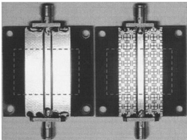
**Figure 2** Fabricated FW-CBCPWs: Non-UC-PBG (left) and UC-PBG (right). The dotted area (20  $\times$  30 mm) was measured
