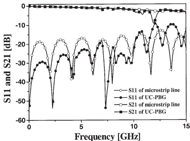
**Figure 5** Measured  $S$ -parameters of the conventional microstrip line and the UC-PBG FW-CBCPW
