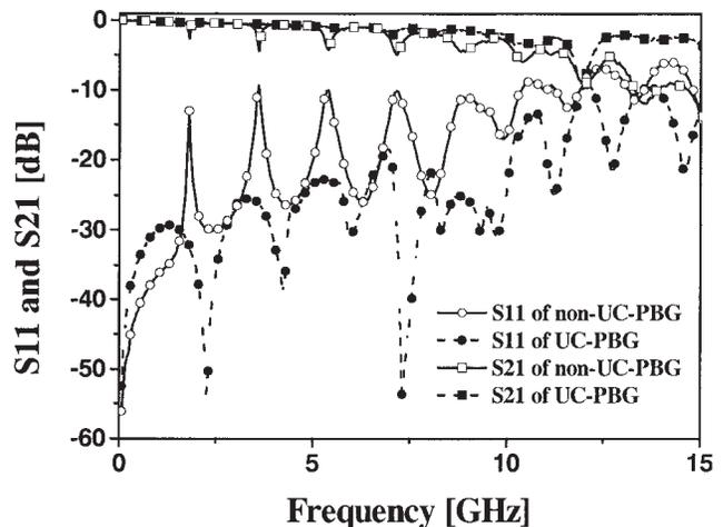
**Figure 4** Measured  $S$ -parameters of the non-UC-PBG and UC-PBG FW-CBCPWs
