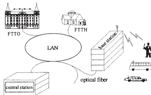
**Figure 1** Distribution network of optical and MMW signals
