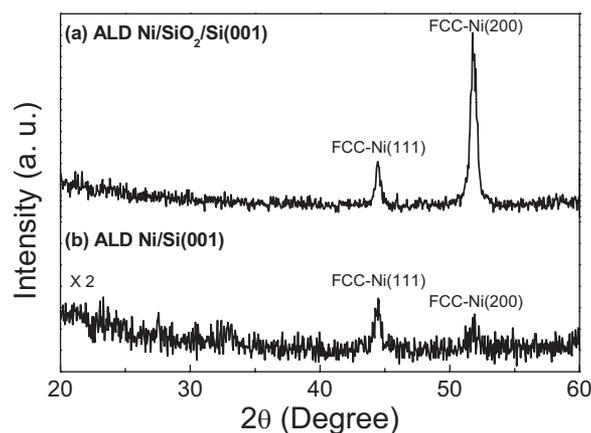
**Figure 4.** SRXRD patterns of 30 nm thick Ni films grown on (a) SiO<sub>2</sub> and (b) Si (SRXRD, Pohang Acceleration Laboratory, 3C2 beam line).
