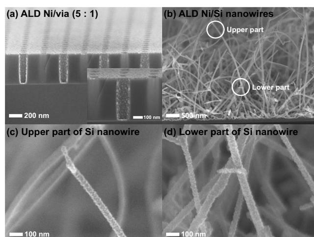
**Figure 5.** FE-SEM images of the ALD Ni films on (a) a nanosize via hole pattern with an aspect ratio of 5:1 (inset: magnified image), (b) Si nanowire, (c) upper, and (d) lower part of the Si nanowire.
