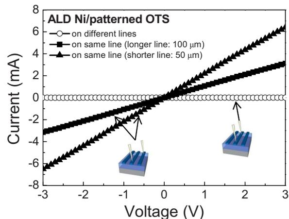
**Figure 8.** (Color online)  $I$ - $V$  measurements of AS-ALD Ni on different lines ( $\circ$ ), same line with 100  $\mu\text{m}$  distance ( $\blacksquare$ ), and 50  $\mu\text{m}$  distance ( $\bullet$ ). (Inset: drawings showing probes on Ni lines.)
