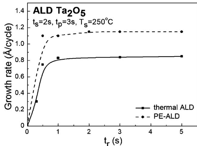
**Figure 2.** Growth rates of thermal and PE-ALD  $\text{Ta}_2\text{O}_5$  as a function of water and oxygen plasma exposure time ( $t_r$ ) on Si(001) substrate at  $T_s = 250^\circ\text{C}$ .
