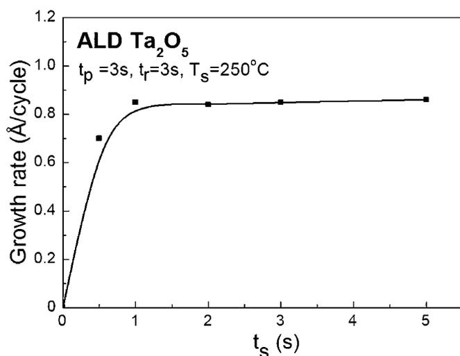
**Figure 1.** Growth rates of thermal ALD  $\text{Ta}_2\text{O}_5$  as a function of PDMAT exposure time ( $t_s$ ) on Si(001) substrate at  $T_s = 250^\circ\text{C}$ .
