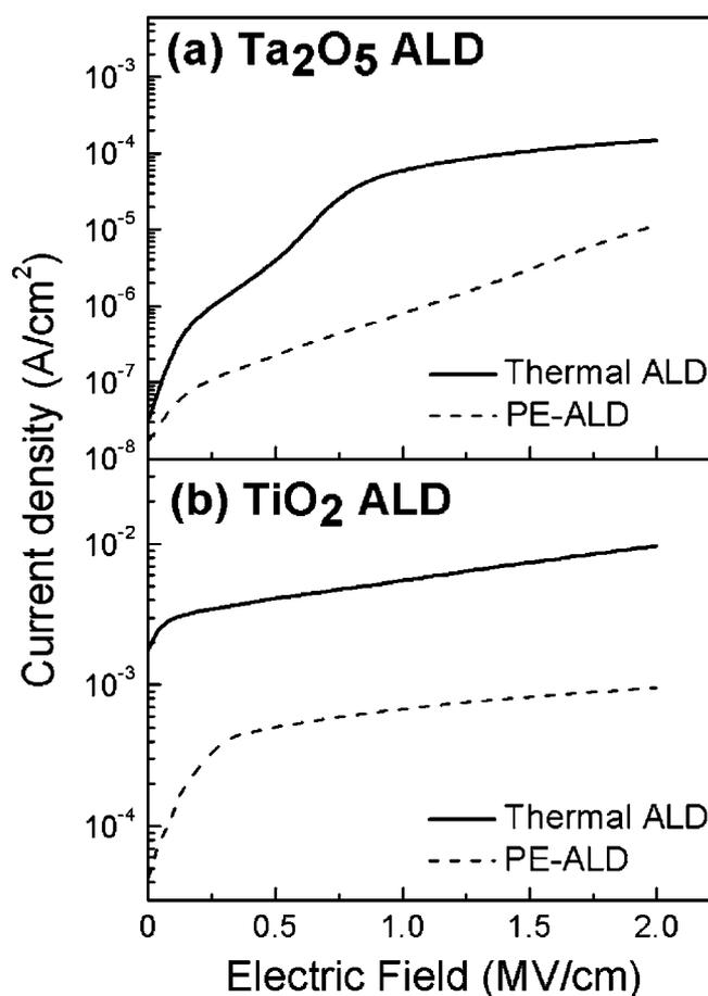
**Figure 5.** Leakage current densities vs electric fields of thermal and PE-ALD (a)  $\text{Ta}_2\text{O}_5$  and (b)  $\text{TiO}_2$  thin film. The film thickness was 10 nm for all films, and the growth temperatures were  $250^\circ\text{C}$  for  $\text{Ta}_2\text{O}_5$  and  $200^\circ\text{C}$  for  $\text{TiO}_2$ , respectively.
