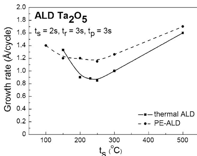
**Figure 3.** Growth rates of thermal and PE-ALD  $\text{Ta}_2\text{O}_5$  as a function of growth temperature  $T_s$ .
